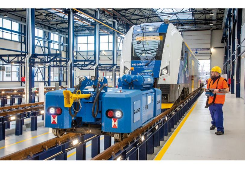
In 2021, a sanitary facility was put into operation in Klatovy, which enables year-round water management services (water replenishment, waste tanks emptying) for various types of trains. Klatovy is an important starting point and destination of, for example, the Berounka express trains. The installed equipment allows the operation of not only express trains, but also Regionova, RegioPanter and other units.
